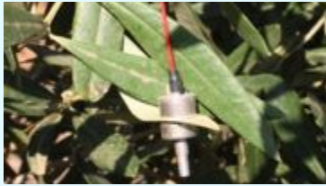
Figure 1. ZIM-probe clamped to a leaf.
