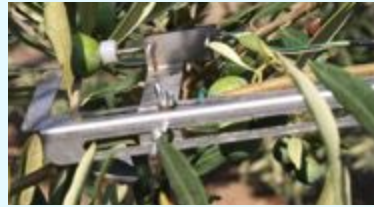
Figure 2. Fruit gauge attached to a fruit.
